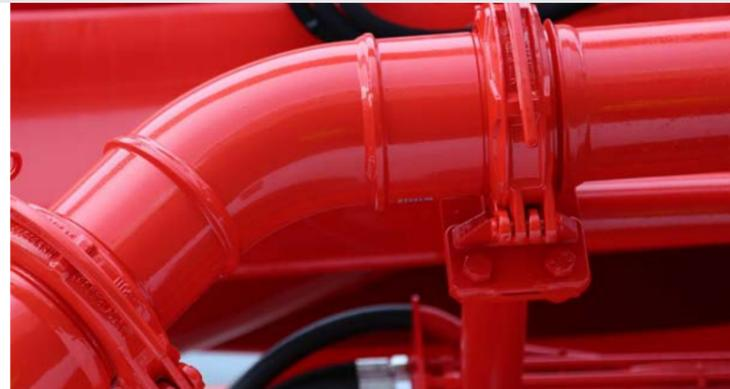
Maintenance-free components reduce operating and maintenance costs, for example thanks to wear-optimized standard elbows with long joints for maximum delivery line service life.
