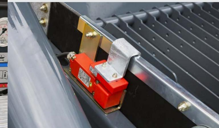
**Agitator safety shutdown via RFID** (Radio Frequency Identification): A detection system using electromagnetic waves, including start-up protection, ensures optimum safety for machine operators.
