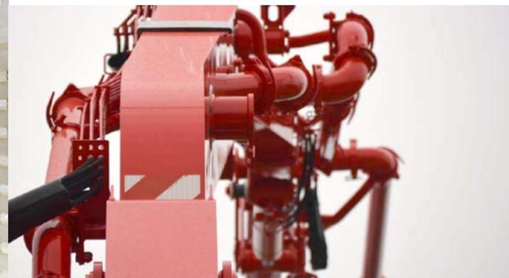
The improved boom hydraulics conserve valuable resources and hydraulic fluid. The optimized response characteristics of the boom, on the other hand, save valuable working time, as it is ready for use more quickly.
