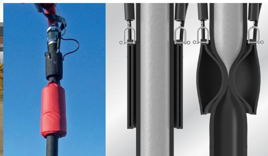
The 46-5 has less horizontal reach but allows a higher boom tip load. This means that an end hose squeeze valve (EQV) and a divided end hose can be used.
