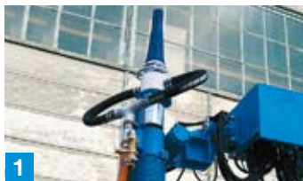
1 Modified MEYCO spraying head for 80 mm hoses and all required nozzle angles.
