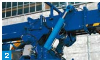
2 Ingenious construction allowing boom to be easily retracted for transport and extended for spraying.
