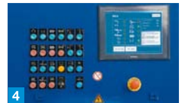
4 Control panel with GUI, positioned near the nozzle-man/operator.
