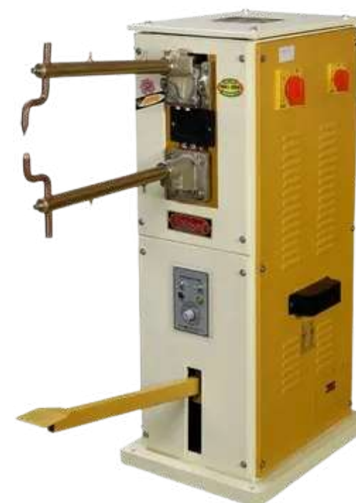
SPOT WELDING QTY-02
